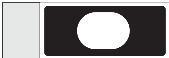
Figure 74 Standard 25 mm x 75 mm x 1 mm slide used during the manufacturing of 17 x 24 mm oblong, single well fluorescent particle slides.
